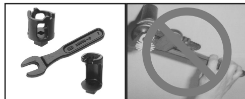
CORRECT (Special installation wrenches) INCORRECT (Designated wrench not used)
